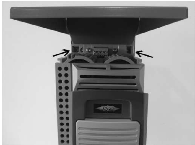
Secure IP21 cover additionally using the screws included in the kit.
