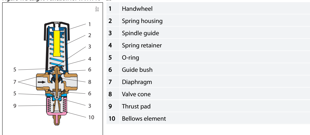
Figure 1: Design / Function for WVFX 10 – 25
