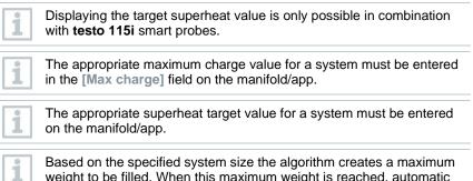
Based on the specified system size the algorithm creates a maximum weight to be filled. When this maximum weight is reached, automatic filling is paused and must be restarted. This prevents overfilling or incorrect filling.
