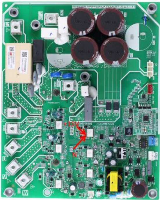
Figure 4-4.10: P N +15V Terminal -+15V IC4/5/6PIN12 ; N- (IC/4/5,6) PIN13
