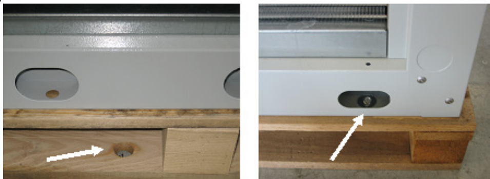
Fig. 7 Special positions of pallet fixing screws
