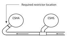
The 1-3/8" restrictor is used for SM115-125 units, the 1-5/8" restrictor is used for SM175-185. The restrictors are supplied with the compressors. The use of a restrictor is not necessary when CSHA is installed in first upstream position or all compressors in the manifold set are CSHA models.
