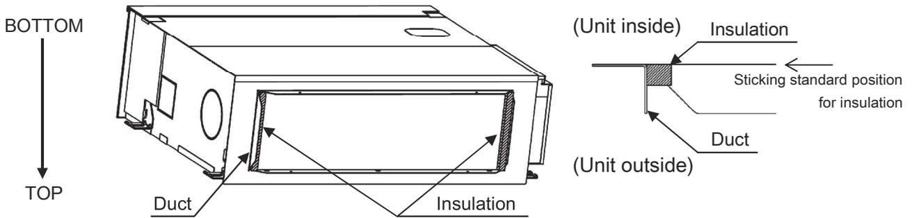
(\*) After unpacking, bottom side of the unit is located at the upper side.
