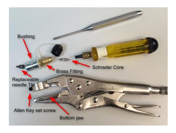
Remover the Schrader core from inside the brass fitting using a Schrader core removal tool (For example the REFCO A-32000).
