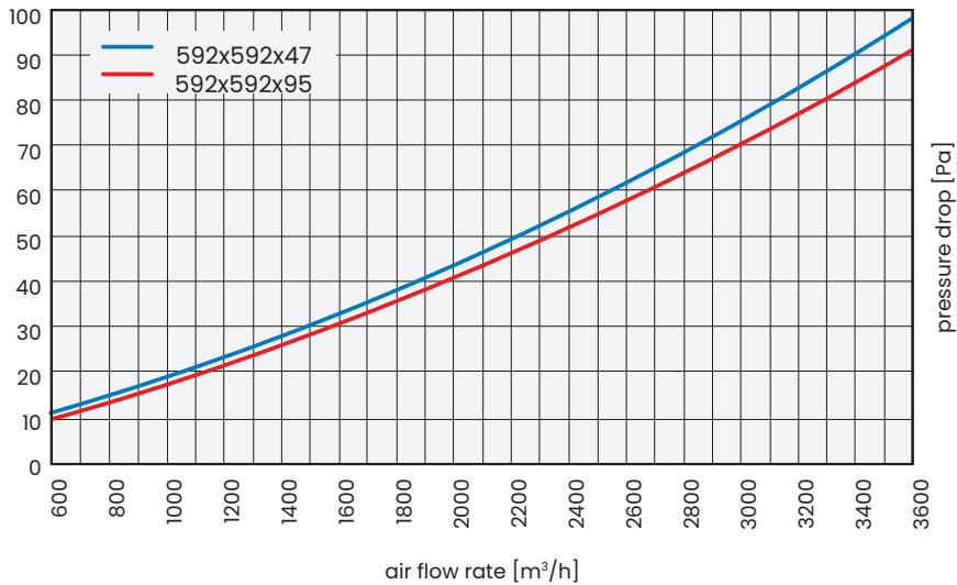
Pressure loss as a function of flow rate for UltraPac 6 filters
