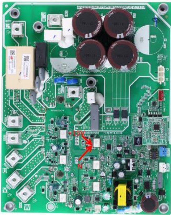
Figure 4-4.10: P N +15V Terminal -+15V IC4/5/6PIN12 ; N- (IC/4/5,6) PIN13
