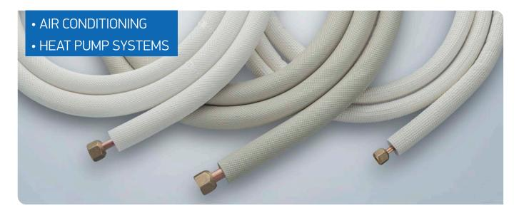
TALOS® ACR Linesets are designed especially for the split Air Conditioning and Heat Pump Systems products requiring installation with flared connections. The unique advantages offered by TALOS® ACR Linesets, including, copper resistance and durability, high performance foam insulation and pre-flared ends with mounted flare nuts, result in significant energy savings and in quick, cost effective field installations.
