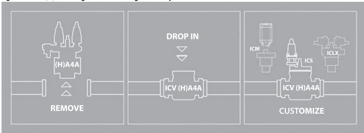
Figure 53: ICV (H)A4A flanged valve housings assembly
