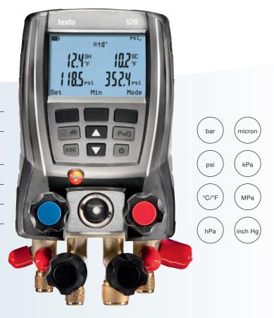
The digital manifold testo 570 is a robust tool for all imaginable measurements on a refrigeration system or heat pump. The instrument is capable of considerably more than just measurement. Pressures, temperatures, vacuum or current – testo 570 analyses them all. It stores all measurement data, right from commissioning, to service and maintenance, through to the error analysis of a system.
