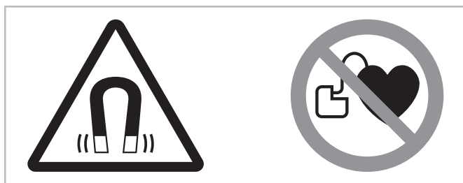
Fig. 21: Warning and prohibition signs on a compressor with permanent magnet motor
