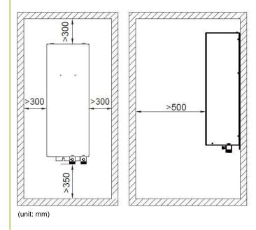
The backup heater is designed to be wall mounted in indoor locations only.
